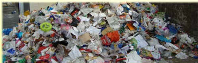
RDF as produced through the standard production line
