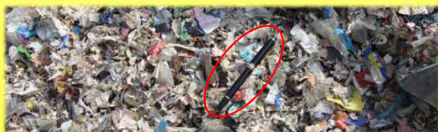
Shredded RDF 40 mm (indicative size of the pen)
