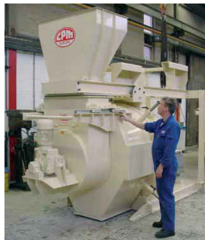
Figure 2.X: Press roller pelletizer (working concept) Figure 2.X: Press roller pelletizer (photo)
