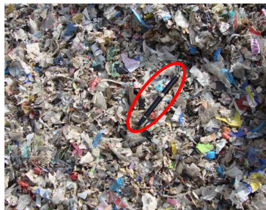
Picture 2.2: Shredded RDF (40mm)
