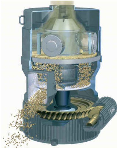
Figure 2.X: Flat die pelletizer (working concept) Figure 2.X: Flat die pelletizer (photo)
