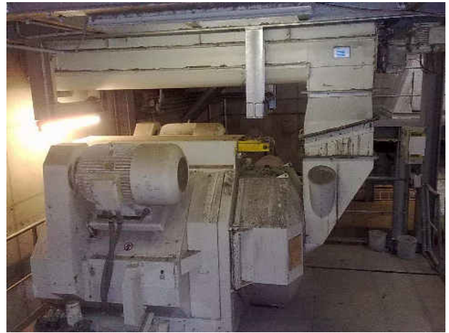
Figure 2.X: Press roller pelletizer (photo)
