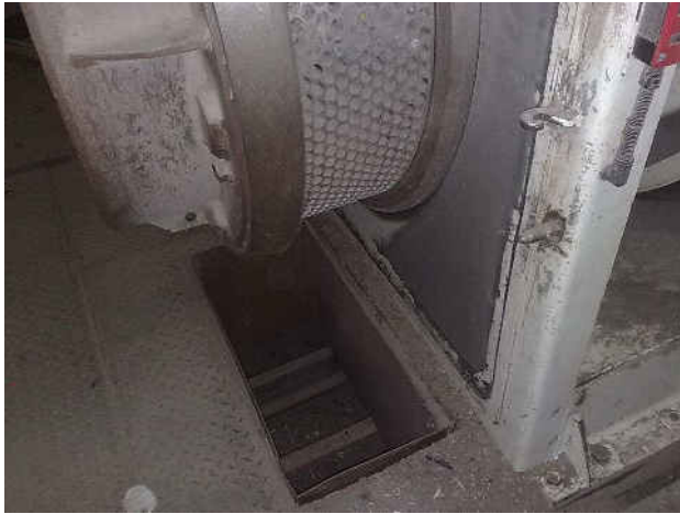
Figure 2.X: Press roller pelletizer (photo)
