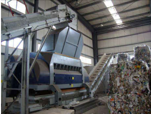
Picture 3.1: RDF shredder
