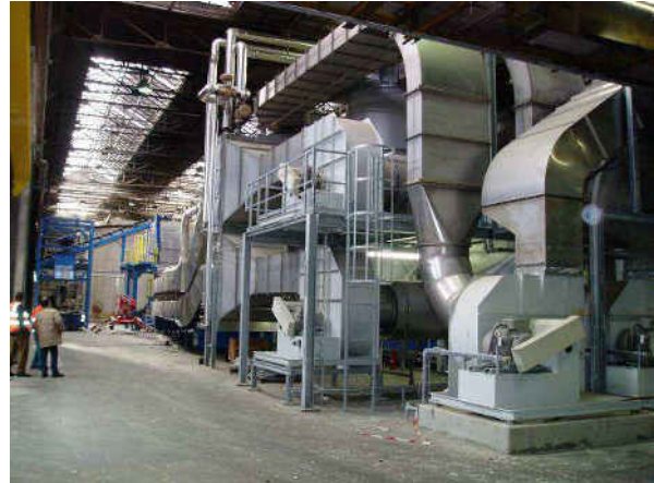
Picture 4.1: RDF air dryer
