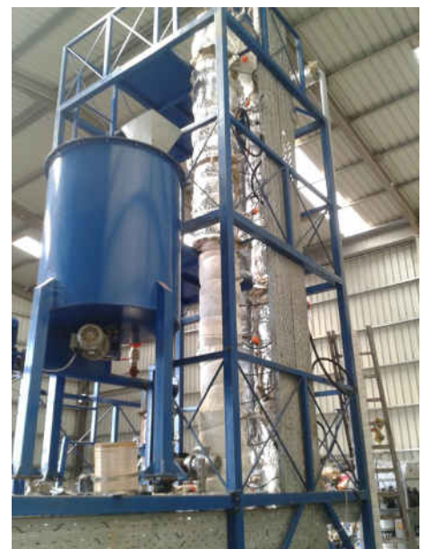
Image 1. Circulating fluidized bed gasifier.
